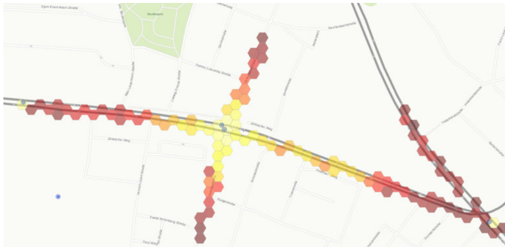
Figure 179 - Distance measurements at an intersection for non-hopping ITS-G5 messages from roadside stations.
