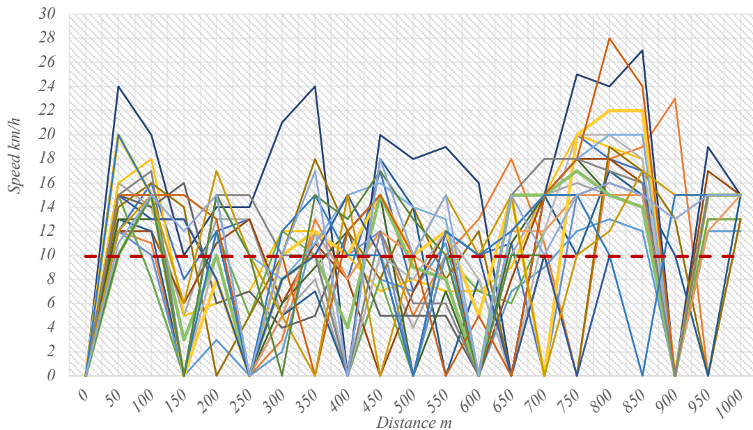
Figure 133 - Speed profiles from the test drives without GLOSA (from KN228 to KN19) (Source: LSBG)
