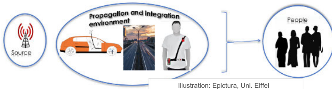
Figure 206 - The three predominant parameters for exposure assessment, namely: (i) EM sources characteristics, (ii) Propagation environment and system integration (close to the body) and (iii) the population to be considered for the exposure.
