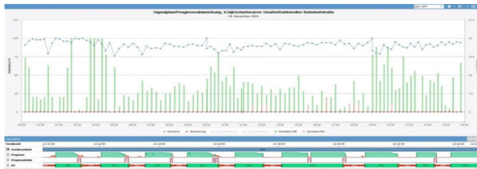
Figure 182 - Forecast accuracy of signal group K3 at junction 1989 on 28.11.2021.
