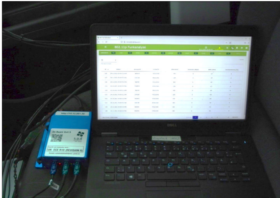
Figure 170 - GLOSA with ETSI ITS G5 communication test system – V-ITS-S equipment for the receiving of MAPEM and SPATEM
