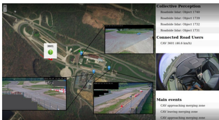
Figure 199 - CAV approaching the lane merging and detection from roadside infrastructure
