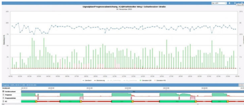
Figure 181 - Forecast accuracy of signal group K2 at junction 1989 on 28.11.2021.
